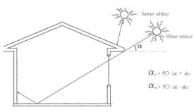
In summer the sun is higher, allowing heat from sunlight to be shaded by a properly sized overhand. In winter the sun is lower, allowing surlight to enter the space through south-facing windows and provide extra space heating
